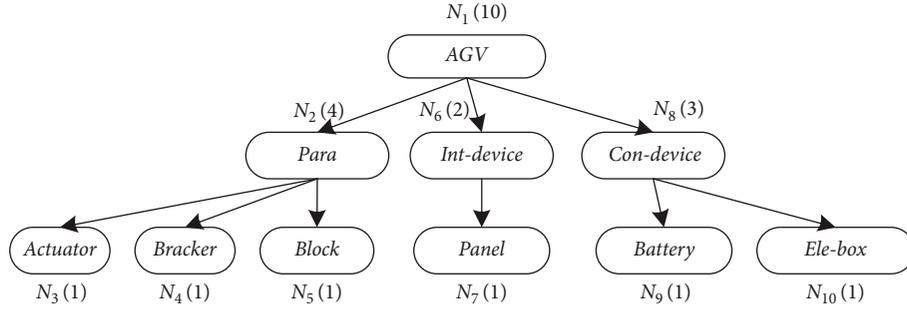
FIGURE 10: Hierarchy of AGV configuration node structure.
