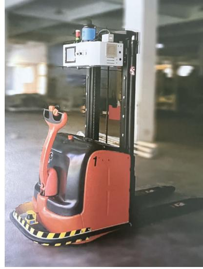
FIGURE 6: The stack-type AGV.
