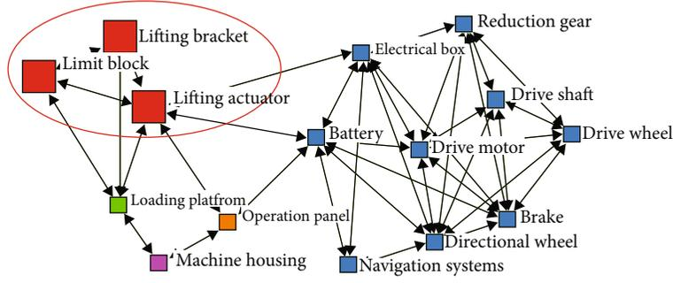
FIGURE 9: The network structure of the AGV.
