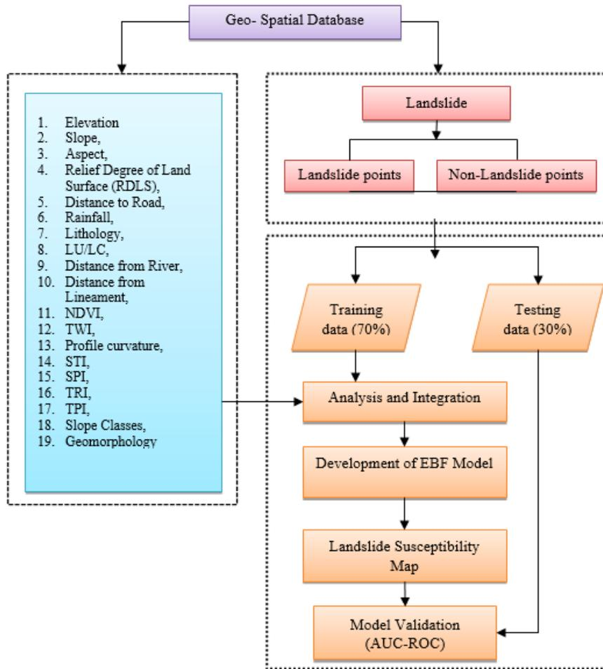
**Fig. 2. Workflow of the methodology**
