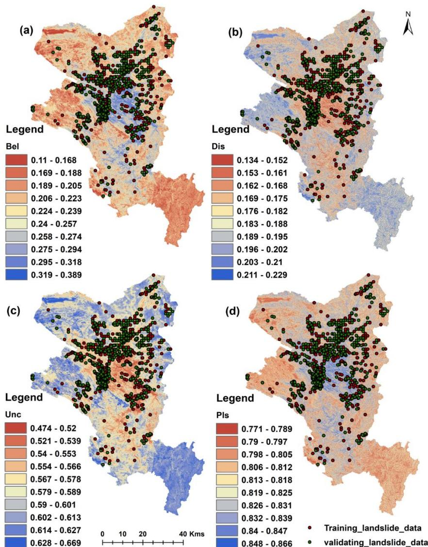
Fig. 3. Integrated results of Evidence Belief Function (EBF) (a) Belief (bel), (b) Disbelief (Dis), (c) Uncertainty (Unc), and (d) Plausibility (Pls)
